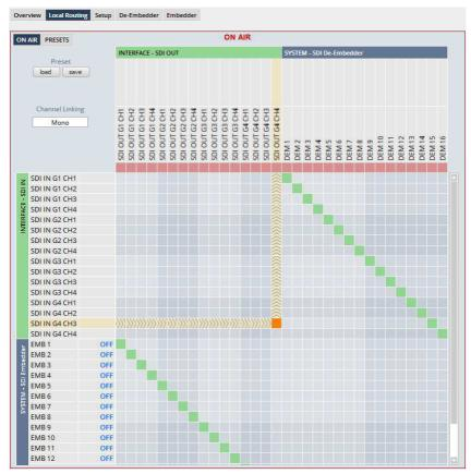
You must use the scroll bar to navigate through the matrix. In the upper left corner you can select between the **ONAIR** and the **PRESETS** view of the matrix.
