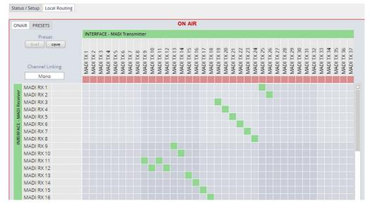
You can also assign device outputs (MAOUT 1 ... MDOUT 16) to MADI transmitter channels For better visibility the matrix has been divided by cutting off the middle part:
