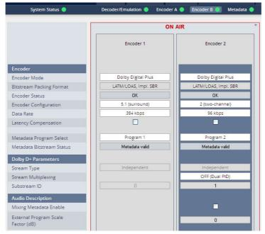
The **OEM** module from Dolby called **CAT561**. The implementation for the **D\*AP8** platform provides two encoded outputs. Both outputs may have independent consumer formats. If both encoders are set for **Dolby Digital plus** encoding special features like providing associated services (e.g. an extra audio track for visually impaired people, AKA audio descriptive service - AD) are available.
