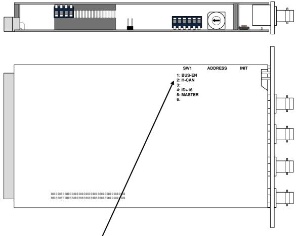
As a new feature you see the **CAN-H** switch above. That allows the module to operate with 1Mbit/s CAN-bus speed. This speed enhancement is helpful if you must log multiple programs from multiple **C8492s** in a compact 64 or compact 256 frame.
