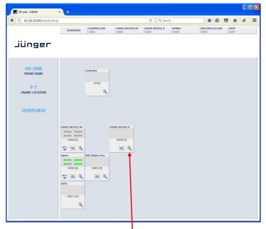
By simply clicking on the spanner tool symbol • you will be forwarded to the control pages of the **C8306** and the status pane on the left hand side, which is also shown on mouse over.
