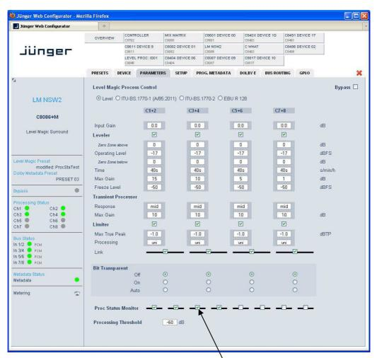
The monitoring of the processing status may be turned **(ON / OFF)** via the respective check boxes: **"Proc Status Monitor"** above. It is important to turn it off if a processing channel is not in use or the leveler max gain settings are too low for good reasons so it will cause an error by definition. This will prevent the system from generating unfounded alarms (if the bad condition is monitored by an external entity).
