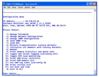
You will get a similar window that shows the momentary IP configuration and a Configuration Menu. The layout depends on the screen settings and the OS. The content of that menu may vary depending on the **Frame Controller** firmware version.
