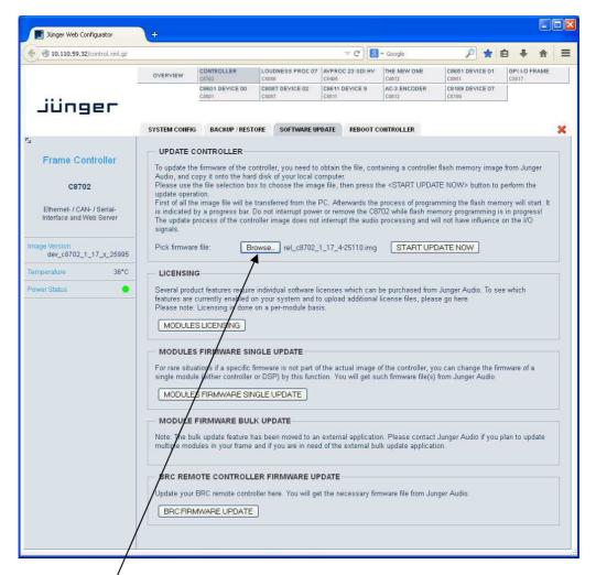
You must browse for the appropriate image file from the previously unpacked ZIP. Once done you must press the **START UPDATE NOW**> soft button. This process has 3 steps. The controller will upload the image file from the **PC** into its memory, afterwards it will erase the flash memory and finally burn the new image file into it.
