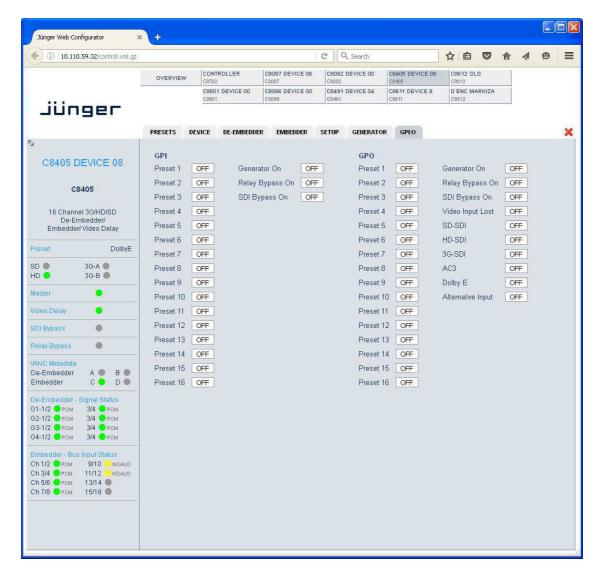
Generator enabled The video generator may be enabled here. The video format it
