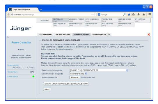
This is a basic tool and it needs a bit of care when using it. You must update module by module and for each module you must choose the respective part of the firmware, all one by one.
