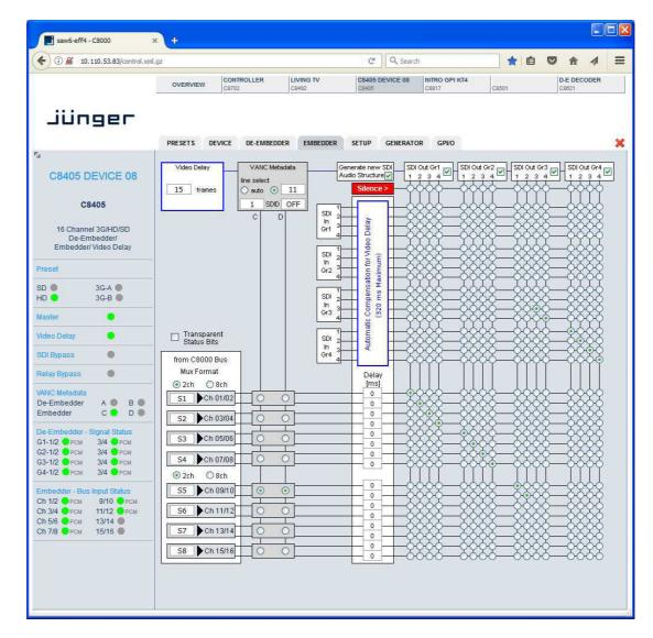
The **EMBEDDER** page is a little more complex because it allows routing within the SDI domain as well as in any combination with signals returned from the audio busses.
