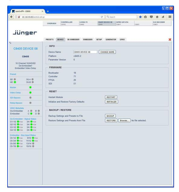
On the **DEVICE** page you can assign a **16 digit name** to the module, perform a warm start by pressing **<RESTART>** or initialize the module to factory default settings by pressing **<INITIALIZE>**.
