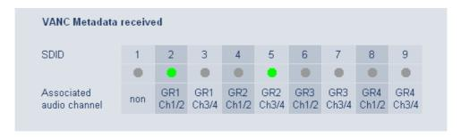
Via the VANC de-embedder routing you may link the respective Metadata to their audio channels. The Junger Audio Metadata system inside the c8k frame makes use of the ASE User Bits to move Metadata to other modules. If you disable the VANC routing these User Bits are transparent again and carry the information from their source somewhere upstream.
