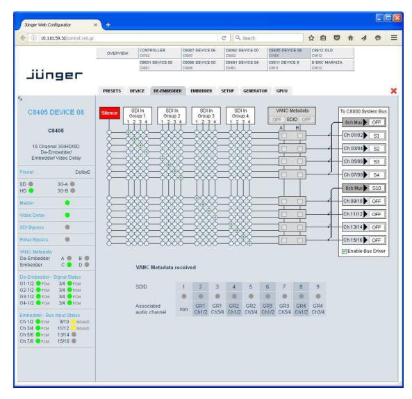
On the **DE-EMBBEDER** page you will get a matrix overview of the signals which are extracted from the SDI data stream and sent to the C8k audio frame bus. The de-embedder can route all of the 16 embedded audio channels in any combination to the C8k audio busses.
