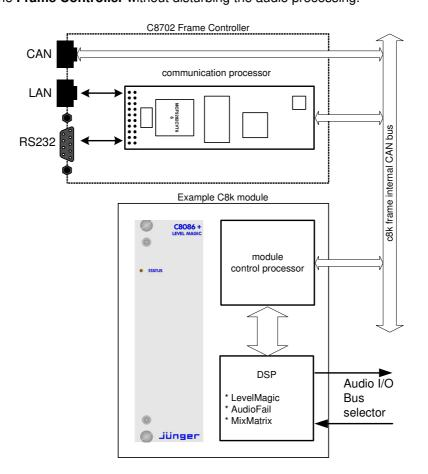
The **communication processor** runs a **HTTP and** an **UDP** server. You may also activate a **Telnet**, an **Ember server** and a **Proxy** to communicate with the **brc** remote controller. As a fee-based option you may activate a **SNMP agent** as well.
