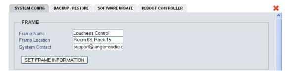
The **Frame Name** and the **Frame Location** as well as the **System Contact** are used by the SNMP **sysObject** OIDs (Object Identifier).
