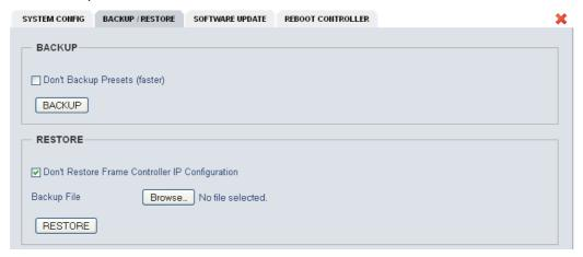
When you press **<BACKUP>** the frame controller will gather all information stored in individual modules of the frame and will build an **XML file** that contains such information. Due to the size of the frame and the complexity of the modules installed it may take a little while. When it's done you will be notified by a pop up. You must select "save file", press **<OK>** and a file dialog will open.
