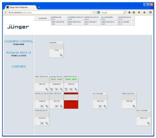
You can only get rid of the **red** coloured module graphic by inserting a working module. If the module is permanently removed you must reboot the Frame Controller. Press the **RESET** button on the front panel briefly, select **REBOOT CONTROLLER** from the web interface or select "**Reboot**" from the console menu. If the reboot was not initiated by the browser you will get a pop up that you have been logged out and you must press the **<OK>** button.
